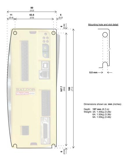
Figure 1 - Mounting and overall dimensions
